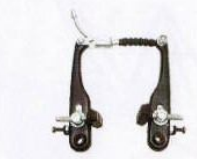
MODEL: BRV-03 BRAKE SET "V" TYPE, CP/PC DIM A: 80-90 MM, DIM B: 28-40 MM DIM L: 116 MM
