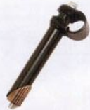
MODEL: HST-18 HANDLE STEM STRAIGHT FOR KID MATERIAL: STEEL BCP/BLACK WITH HEX BOLT STEM DIA: 21.90X 1.6 SWG STEM LENGTH: 135 MM
