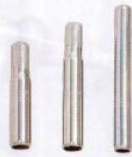
MODEL: MCC - 09 SEAT PILLAR CP/POWDER COATED STEM DIA: 25.4MM NECK DIA: 22.6MM LENGTH & DIA. TO ORDER
