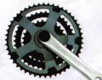
MODEL: CT-08 TRIPLE CWC CL WIDER CP CRANK WITH SPIDER 1/2X3/32 - 28/38/48T CRANK - 170MM
